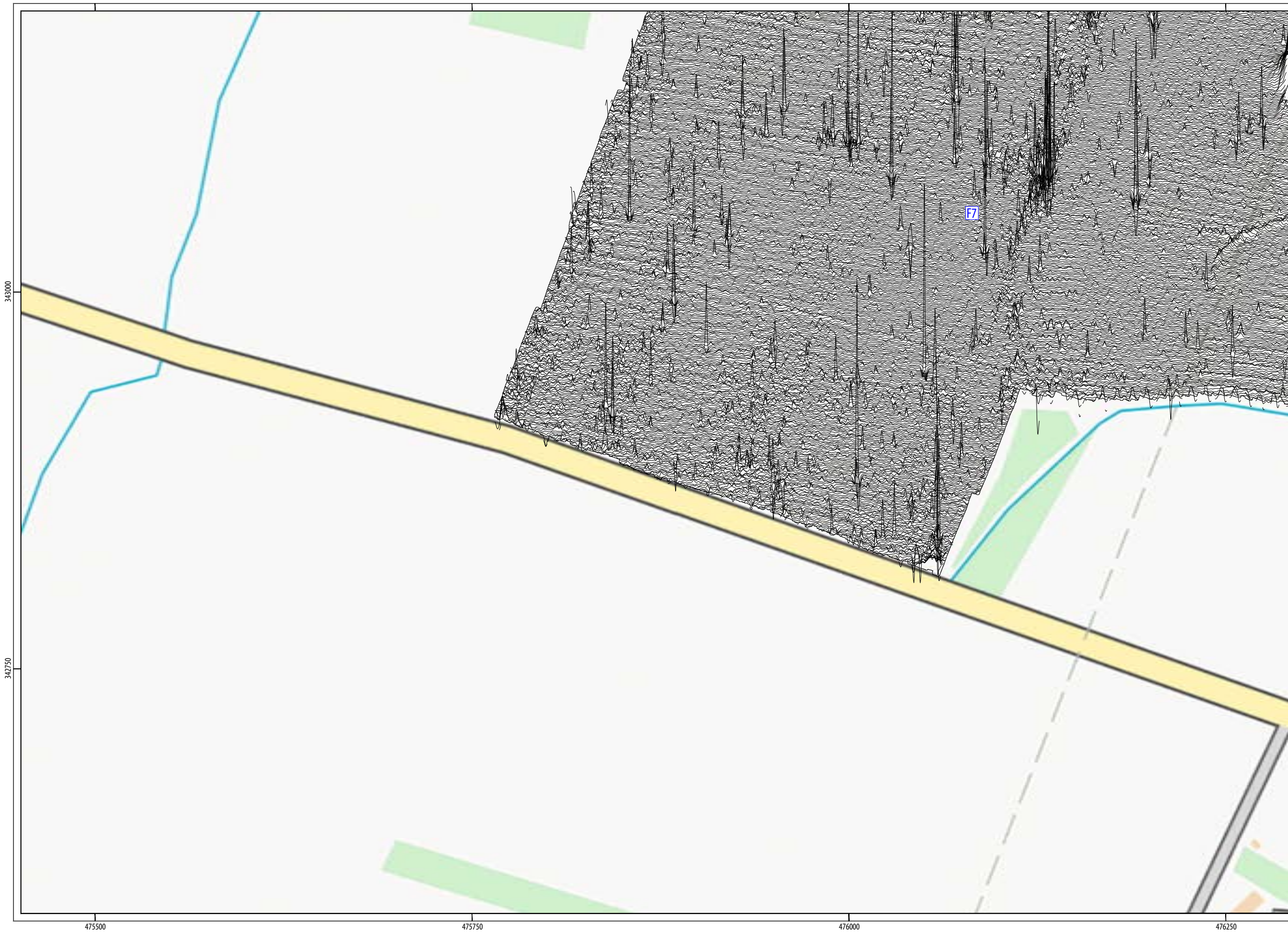
ILLUS 19 XY trace plot of minimally processed magnetometer data; Sector 4
