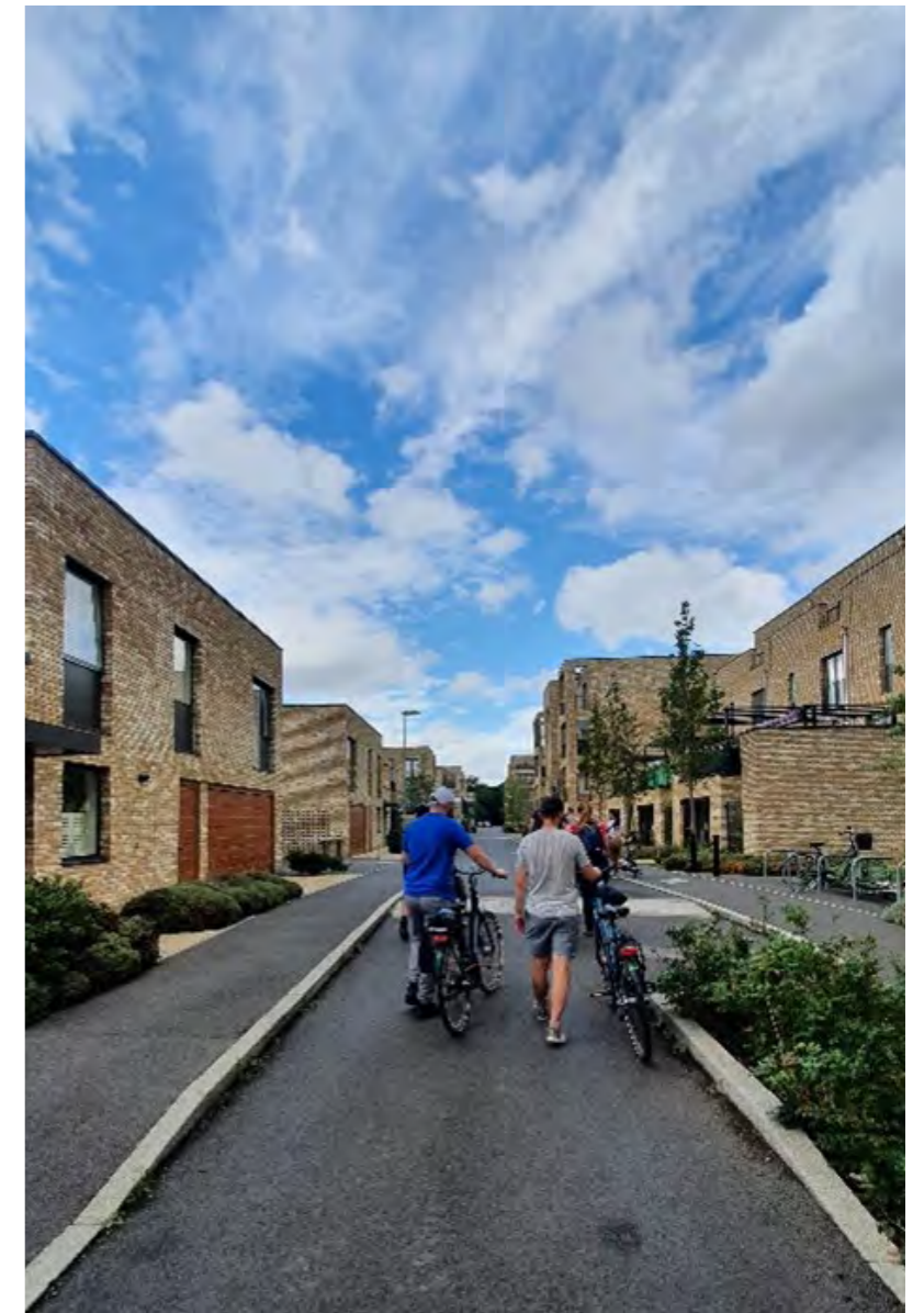
Great Kneighton and Ninewells, Cambridgeshire. Slightly different takes on the conventional residential street. Building line gives continuity and a strong sense of enclosure. Pedestrian priority intervention using a planting area that intentionally narrows the street to disrupt vehicle continuity. The image on the right is an example of how 3-storey house types can enable a wider street section without compromising the sense of enclosure. Here the additional street width allows for the relatively deep liner park alongside the vehicle path and footpath. Note pedestrians feel safe and comfortable to walk in the vehicle path. (Photographs by Rebecca Clark)
