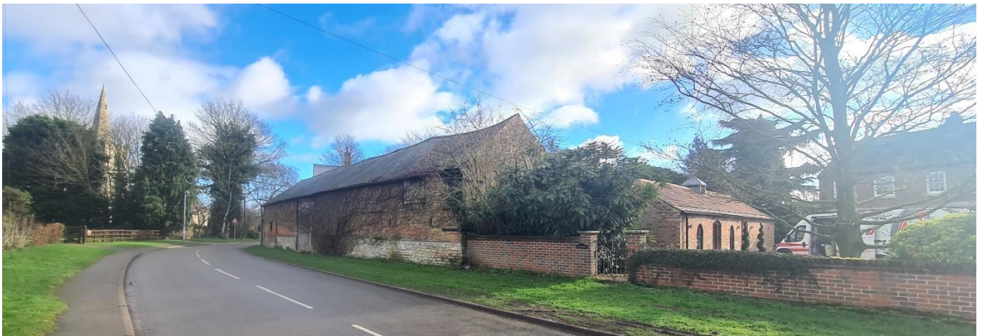
Figure 26 - Traditional barn with stone base, bricks above with its elongated plan form (Grange Farm, Costock Road). Holy Trinity Church visible in the background to the left.
