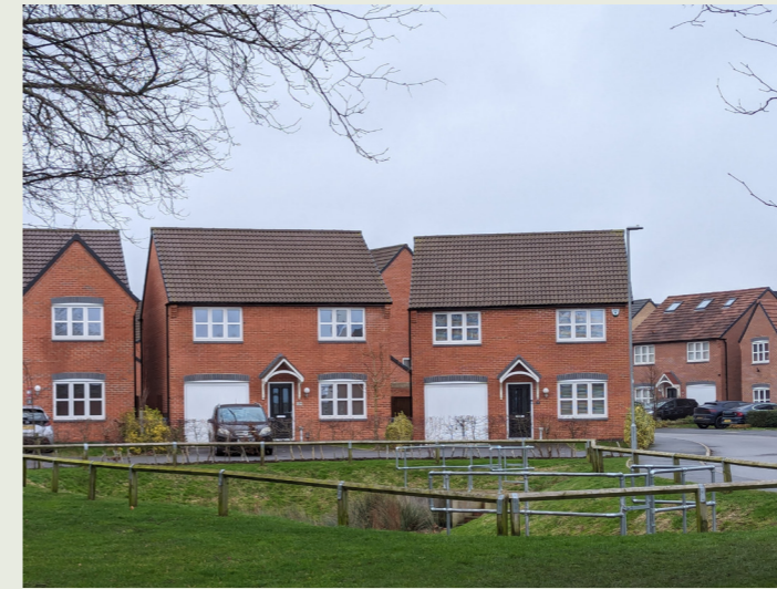
Fig 78: Detention ponds feature heavily at site entrances. Poor integration of SuDS and low value contributions to public space
